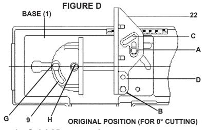
Note: Make sure "C" slot is free of casting flush so the vise can be positioned in all angles.
